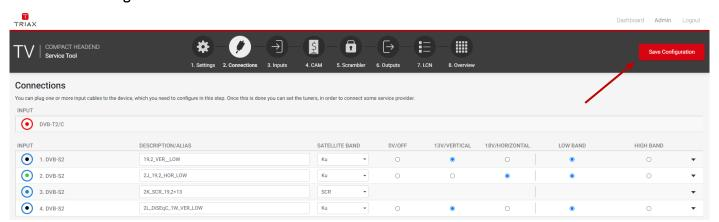
An important button when you change your configuration of the headend system is the "Save Configuration" button placed in the upper right-hand corner of the Service Tool window.
