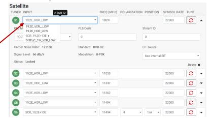
To select the required input / SAT-IF signal, click on the input field to open the drop-down list with the inputs you can choose from.
