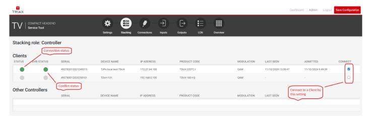
The Controller's Stacking page shows status for clients connected to the controller. It also show unconnected clients, attempting to connect to the controller. A Client can be added to the solution by selecting "Connect" for the given client.
