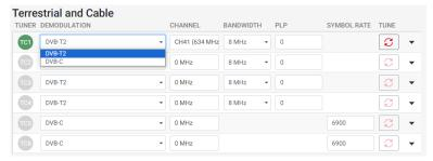
To select the required demodulation, click on the demodulation field to open the drop-down list with demodulations you can choose from.
