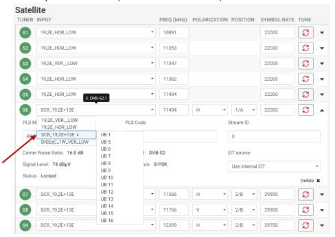
You must select the SCR user band and the Polarisation and Satellite position.
