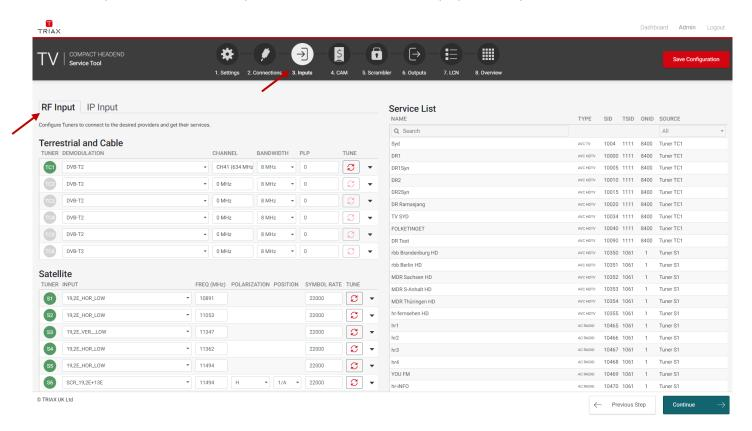
The "Inputs" page shows all RF input tuners. The colour of the tuner number shows the status of each tuner.
