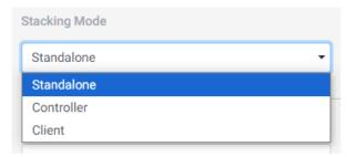
By default the TDcH and TDmH are set to Standalone Mode. This is the legacy mode, where only a single headend unit is deployed. If more units are deployed in a solution, then each unit must be assigned a specific Stacking role. This role is assigned in the Stacking Mode dropdown list. The roles in a stacking solution are:
