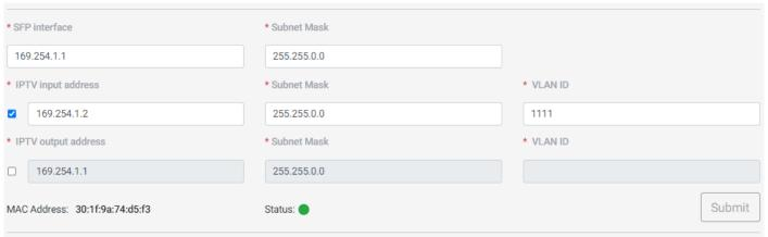
If VLAN is enabled for IPTV output, as in the example shown below, the traffic of any configured IPTV output streams will be tagged by the Headend with the configured VLAN ID (2222).
