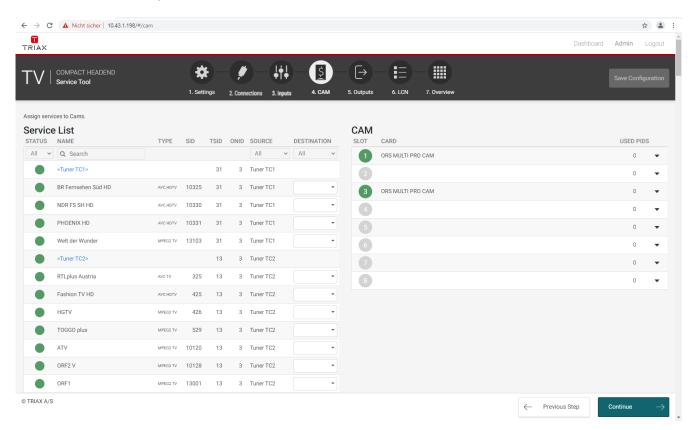
You must configure the CA modules individually. When you open the Configuration window for a CA module in a new configuration, only default values are displayed.
