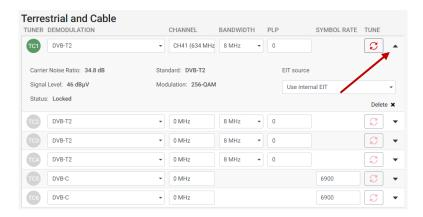
Carrier Noise Ratio: Shows the carrier to noise ratio of the input signal
