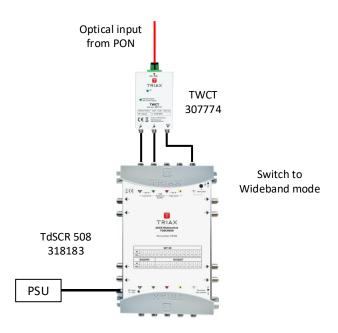
The system can be exteded with additional switches. They must also be switched to Wideband mode
