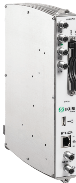
HTI-424 3863 Quad transmodulator with IPTV Receives contents from 4 DVB-T/T2, DVB-S/S2, DVB-C or IPTV transponders/muxes, decrypts and broadcasts them in 4 DVB-T or DVB-C or on IPTV output channels ; 64 IPTV multicast outputs. Double Common Interface.
